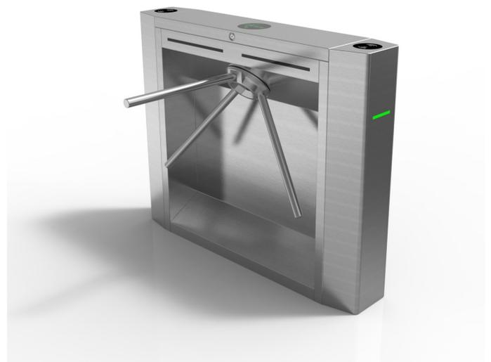
The design of any tripod turnstile means they can be climbed over or crawled under and for this reason they should be installed near a staffed security point.
